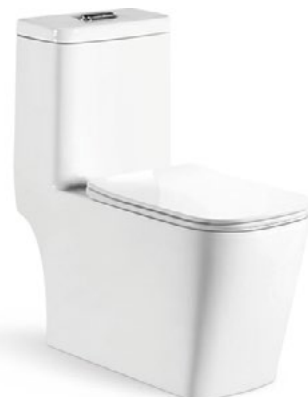
8108 Siphonic one-piece toilet Size: 690x375x775 mm S-trap, 300/400 mm roughing-in
