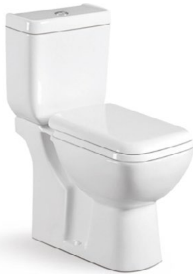
1036A 直冲分体马桶 Washdown two-piece toilet 尺寸 / Size: 680x380x800 mm 墙排 / P-trap, 180 mm roughing-in 地排 / S-trap, 250 mm roughing-in
