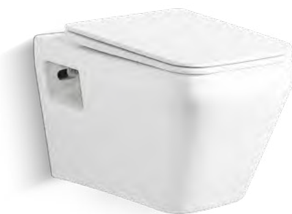
WH-047 挂便器 Wall-hung toilet 尺寸 / Size: 545x360x380 mm 墙排 / P-trap, 180mm roughing-in
