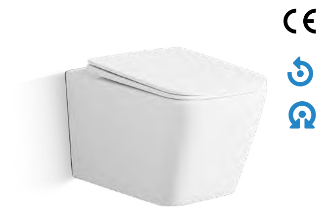
1048W-S 挂便器 Wall-hung toilet 尺寸 / Size: 510x360x350 mm 墙排 / P-trap, 180mm roughing-in Tornado Silent Flush & Rimless Flush
