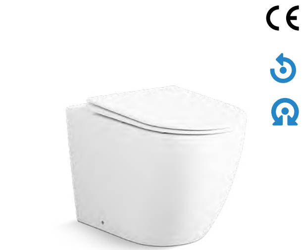
1049FW 直冲落地马桶 Washdown floor mounted toilet 尺寸 /Size: 550x360x400 mm 墙排 /P-trap, 180 mm roughing-in
